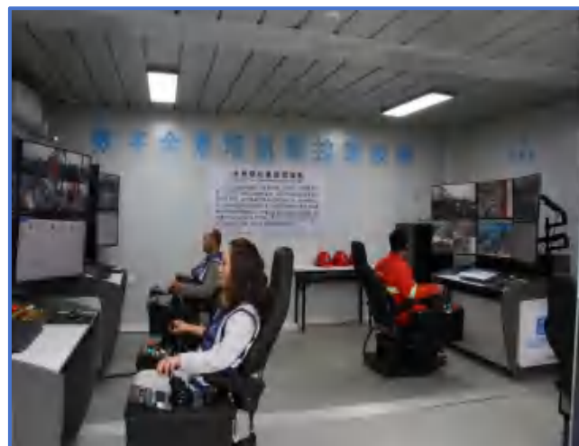
图10-23 5G塔吊集控驾驶舱
